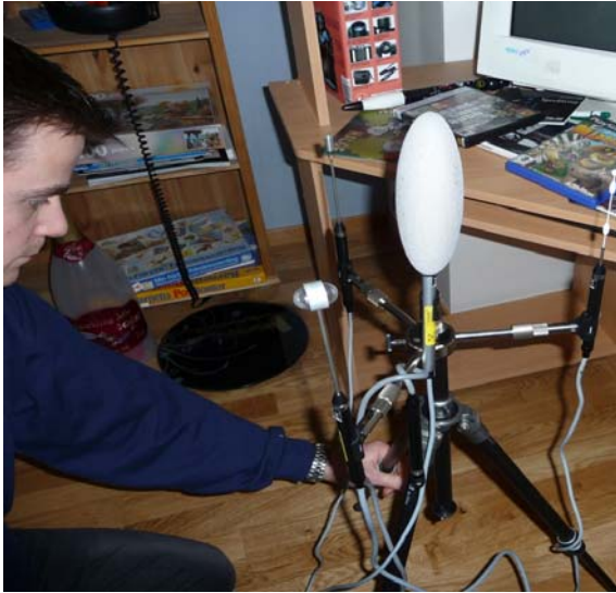
Figure 47 Measuring the operative temperature in an apartment in Brogården, Sweden. (Source: SP)
