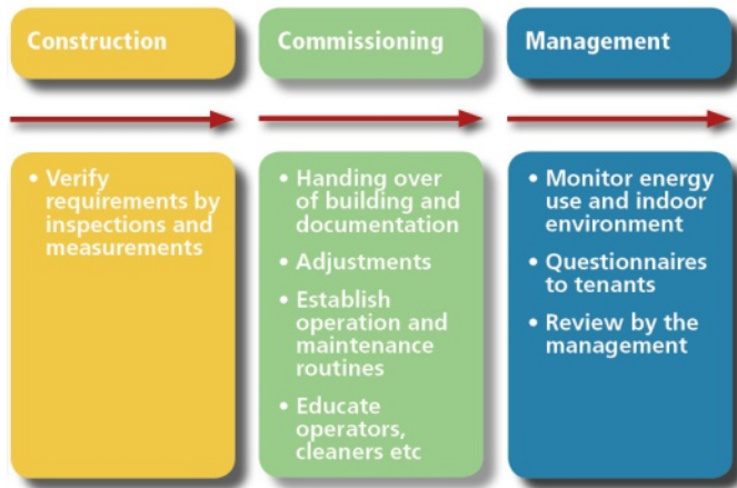
Figure 44 The commissioning process reaches from construction and into the management phase.
