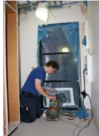
Figure 23 The air tightness of the building envelope was verified using blower door test.
